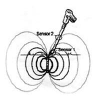
As you can see from the drawing above, the Maghorn has two sensors used to detect the magnetic field of ferrous objects. When sensor 1 is closer to the object than sensor two, the Maghorn's pitch will become higher or more shrill, indicating that it has detected a ferrous object. Experiment with an object above ground or in a known location to become familiar with the Maghorn's sounds and responses.
