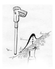
Plastic valve boxes may have a strong magnet inside to make them easy to locate. In this situation you should use caution because the magnet will produce weak signals to each side of the box and a stronger peak signal over the center of the box. (See Sketch in Section 4.2) Turning the sensitivity down as you begin to detect the magnetic marker will help you eliminate the unwanted signals.
