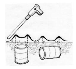
Laying on its side the drum will present two weaker and more seperated peaks while in an upright position the peaks will be closer together and possibly stronger. Most drums can be located up to 8 feet in depth.
