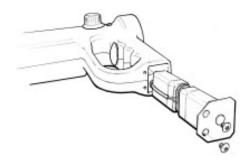
Remove the old batteries and install the new ones in position exactly as the ones you have removed. When replacing your batteries take care to not damage the wires and connector.
